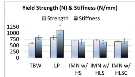
**Figure 3:** Yield strength and stiffness of the Olecranon fixation devices post cyclic testing.
