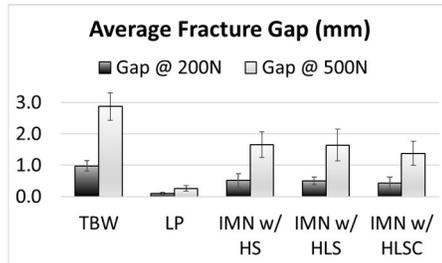
**Figure 2:** Average gapping of the osteotomy during cyclic application of 200 N and 500 N loads.
