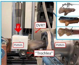
**Figure 1:** Test setup and illustration of Olecranon fixation devices tested.
